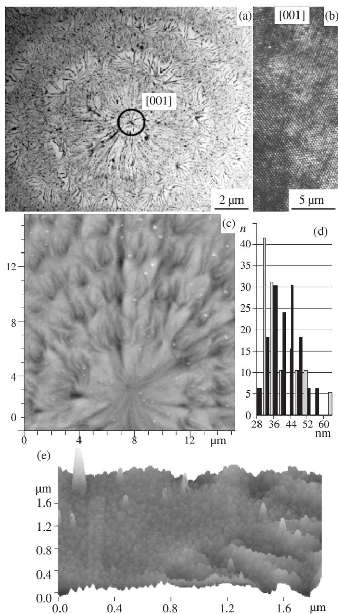
**Fig. 2.** Micrographs of  $\alpha\text{Fe}_2\text{O}_3$  spherulites: TEM (a) indicating  $\sim 90^\circ$  rotation of the unit cell between adjacent bright (perfect, almost single crystalline) and dark (imperfect) concentric zones (with [001] normal and parallel to the film plane, correspondingly), HREM of the spherulite centre (b), AFM (c), globular size histograms (d) for amorphous (gray) and crystal (black) film areas for AFM image of amorphous-crystalline (left-right) interface (e).
