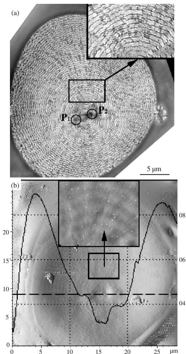
**Fig. 1.** Micrographs of Se spherulite in amorphous matrix with insets of higher magnification: TEM (a) indicating  $60^\circ$  rotation of the unit cell between adjacent dark lines, roughly traces of  $\{100\}$ , AFM (b) with a profile superimposed (measured along the dashed horizontal line).
